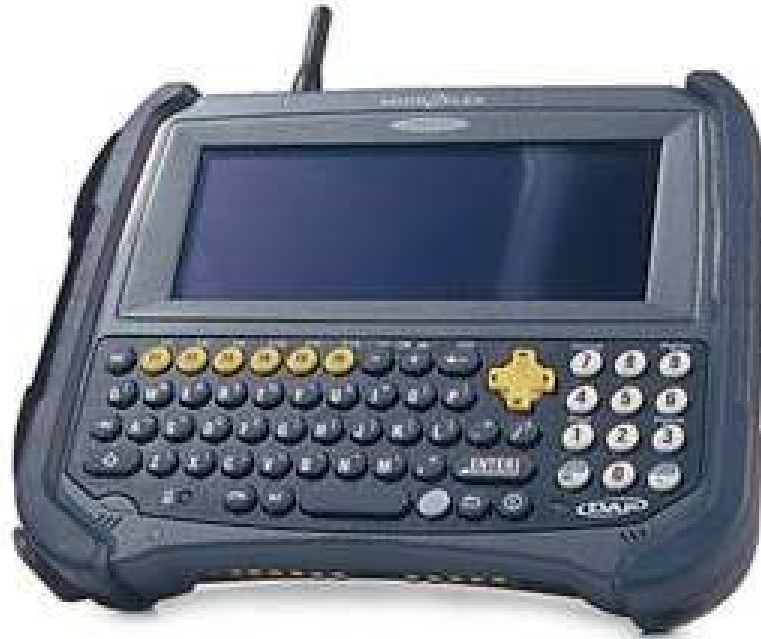
Figure 2: A mobile data terminal in a police patrol car receives instructions from a CAD system via UHF Radio
